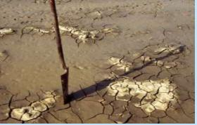
The potential instability of a soil may be measured as its dispersion ratio. Particle-size analysis (PSA) uses a dispersant to deflocculate the clay; performing PSA both with and without the dispersant gives an indication of its inherent structural instability.
